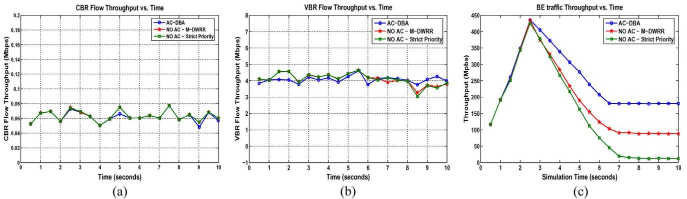
Fig. 6. CoS traffic throughput. (a) CBR flow throughput. (b) VBR flow throughput. (c) BE total throughput.
